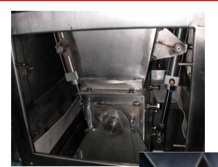
It includes Weighing hopper, Loadcell system, Pneumatic discharge gate and weighing controller etc.
