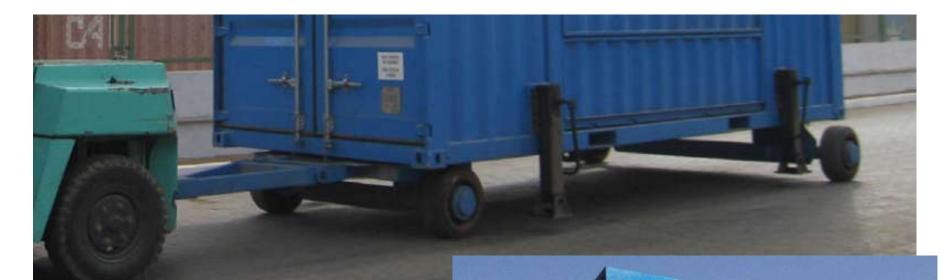
Moving Unit of Towing is mounted beneath the lower containers. It includes tow axle, tow bar and wheels. 2 rear wheels are fixed mounted, and 2 front wheels are mounted on a pivoted axle with tow bar, enable the container system can be moved at quayside by towing.
