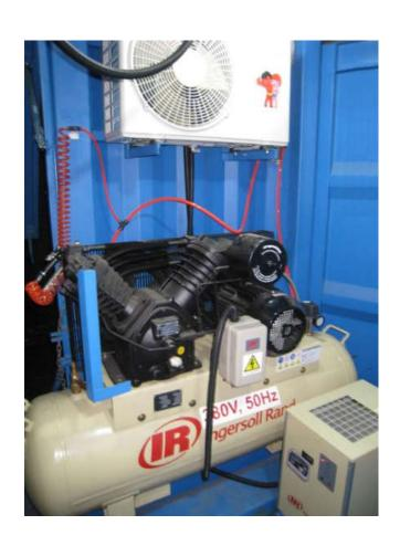
Air Compressor and Pneumatic circuit
