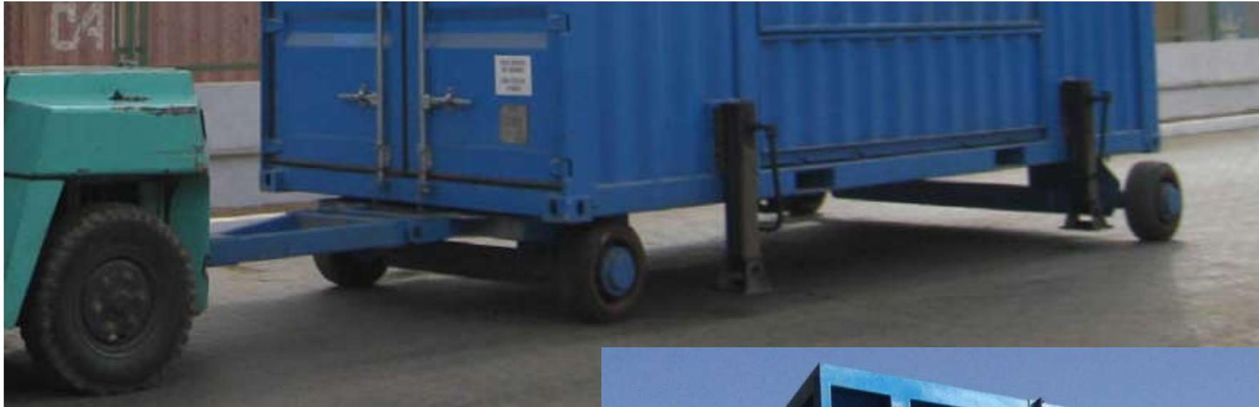
Moving Unit of Towing is mounted beneath the lower containers. It includes tow axle, tow bar and wheels. 2 rear wheels are fixed mounted, and 2 front wheels are mounted on a pivoted axle with tow bar, enable the container system can be moved at quayside by towing.
