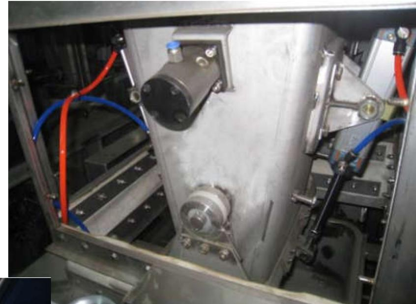
It includes Weighing hopper, Loadcell system, Pneumatic discharge gate and weighing controller etc.
